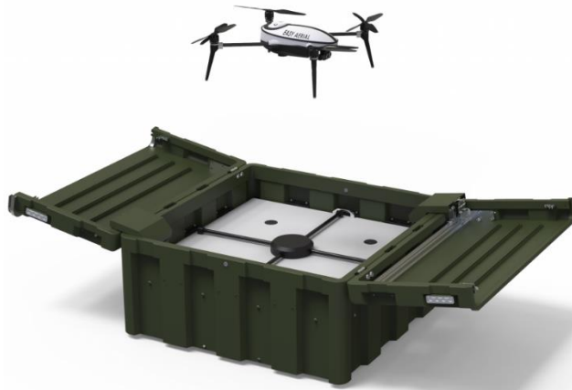
Figure 3: Rendered design of the Drone-in-a-box system
